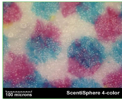
Fragrance microcapsules shown on printed surface
